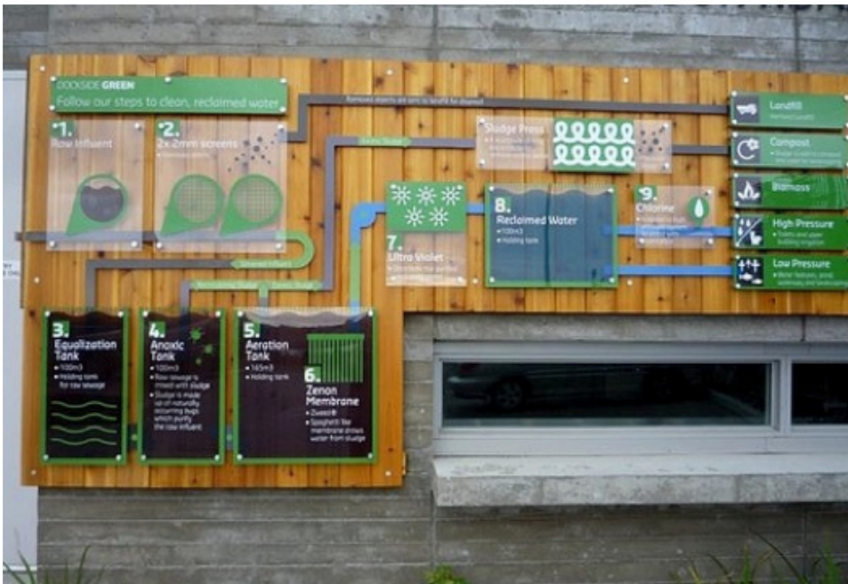
Photo: Example interpretive signage (solarpedia.com)
