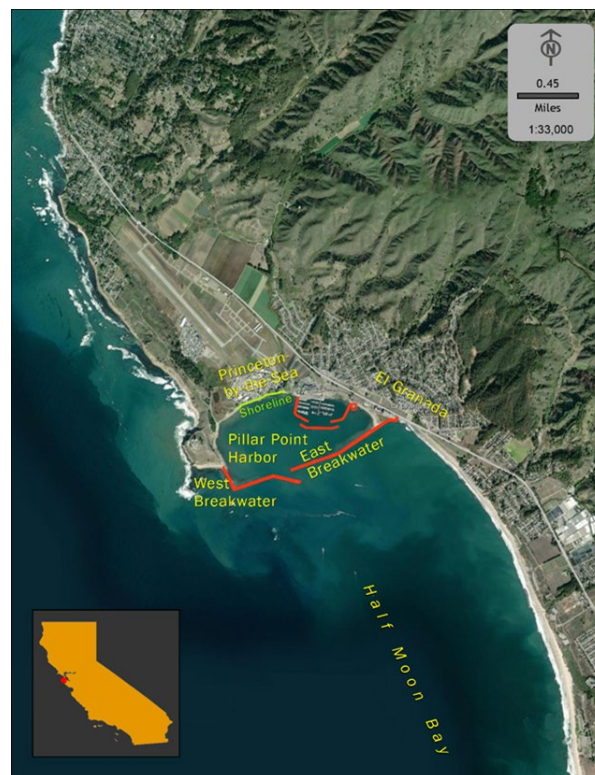
Figure 1. Pillar Point Harbor Federal breakwaters (East and West in red) and inner non-Federal breakwaters (also shown in red), Princeton shoreline (green). Miramontes Point is about a half mile below the bottom of the image.
