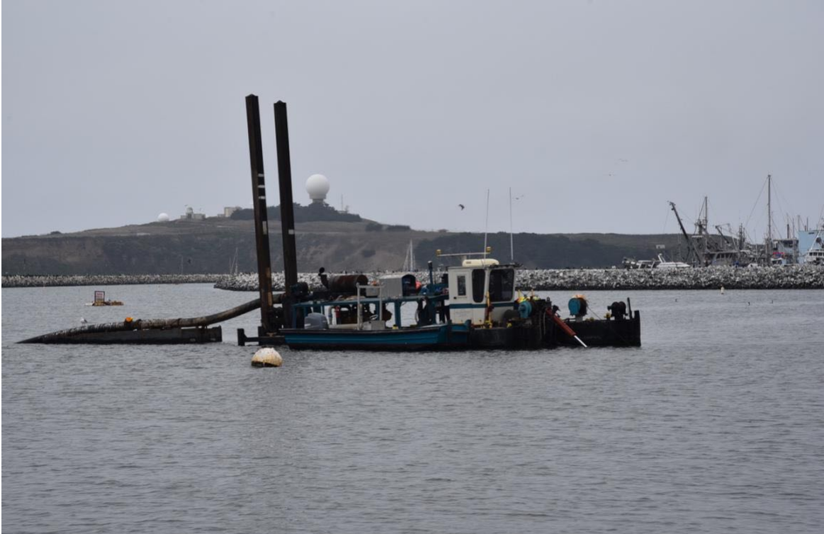
Cutterhead suction dredge #1
