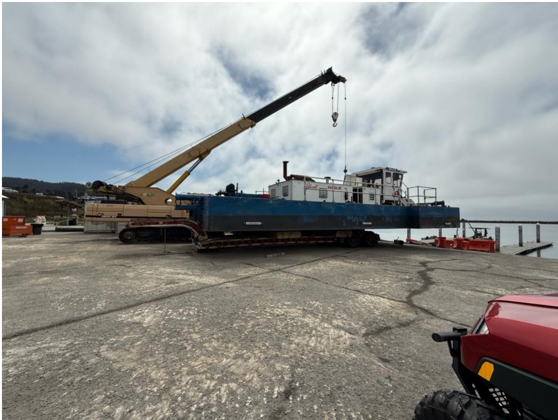
Launching of second dredge for placement of dredged sand at Surfers Beach
