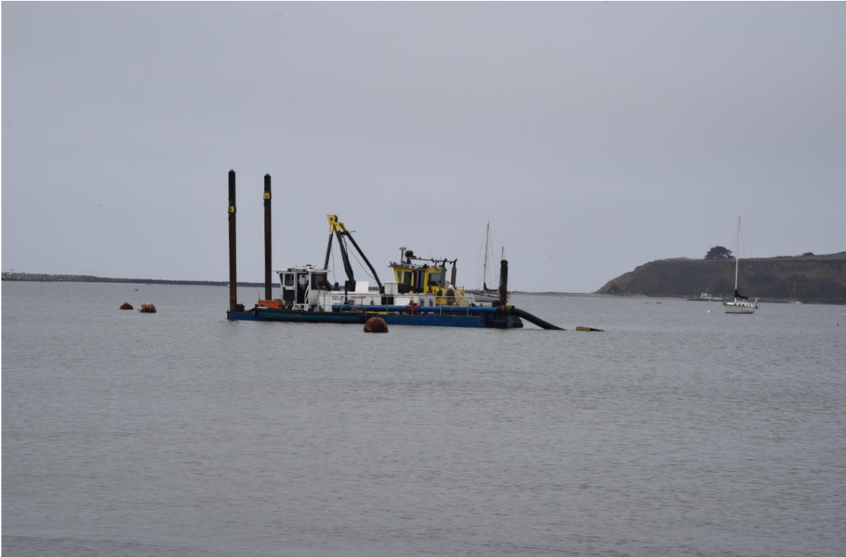
Cutterhead suction dredge #2
